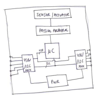
Diagram of a generic Arduino Eslov block
